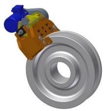
Designed as parking brakes to be applied when equipment comes to a full stop, WB wheel brakes can be also used as dynamic brakes in an emergency situation (e-stop). By applying spring force directly on the wheel flanges, they minimize the amount of stress and strain otherwise placed on sill beams and truck assemblies of a crane.
