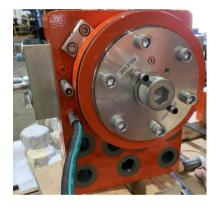
Hydraulic Emergency Brakes are used on the low-speed shaft side of a drive and must provide sufficient torque to overcome a low-speed failure such as a gearbox, coupling, or other transmission failure. They apply braking torque on a disc bolted to the drum flange in order to stop or hold the load.
