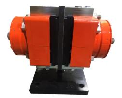
HEB is spring applied and hydraulic released emergency brake. Braking force is directly applied to the brake shoes by a high capacity spring pack. The organic brake friction shoes press on the both sides of a rotating steel disc, providing the friction forces and thus braking capacity. Emergency Brakes are imperative for crane safety.
